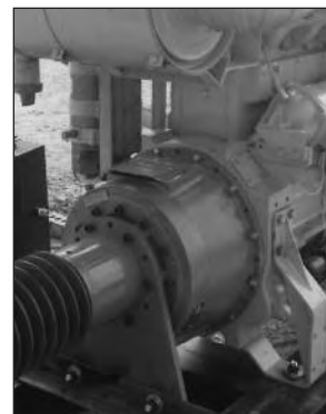
Wichita PTO mounted on Caterpillar diesel engine.
