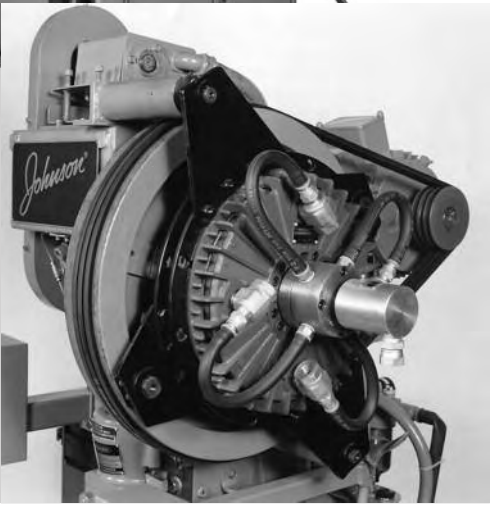
The simple external air system with quick release valves provides smooth, fast cycling.
