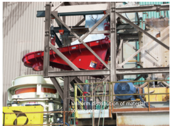
Blended material feeding directly from the Crusher Loading Feeder to the crusher.
