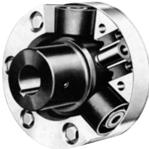
The trunnion pins are fitted into the outer diameter of the hub and welded, thus becoming an integral part of the unit. The neoprene biscuits are pressed over the trunnion blocks, and are retained by snap rings.
