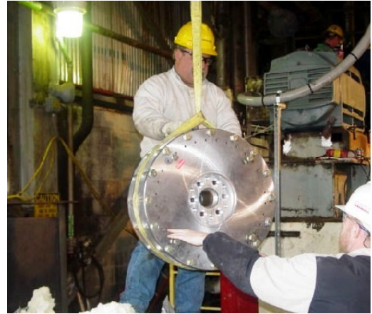
FGC 21.0D, 500 hp 1200 rpm, Pulp & Paper, Debarking Drum, Jay, ME, USA
