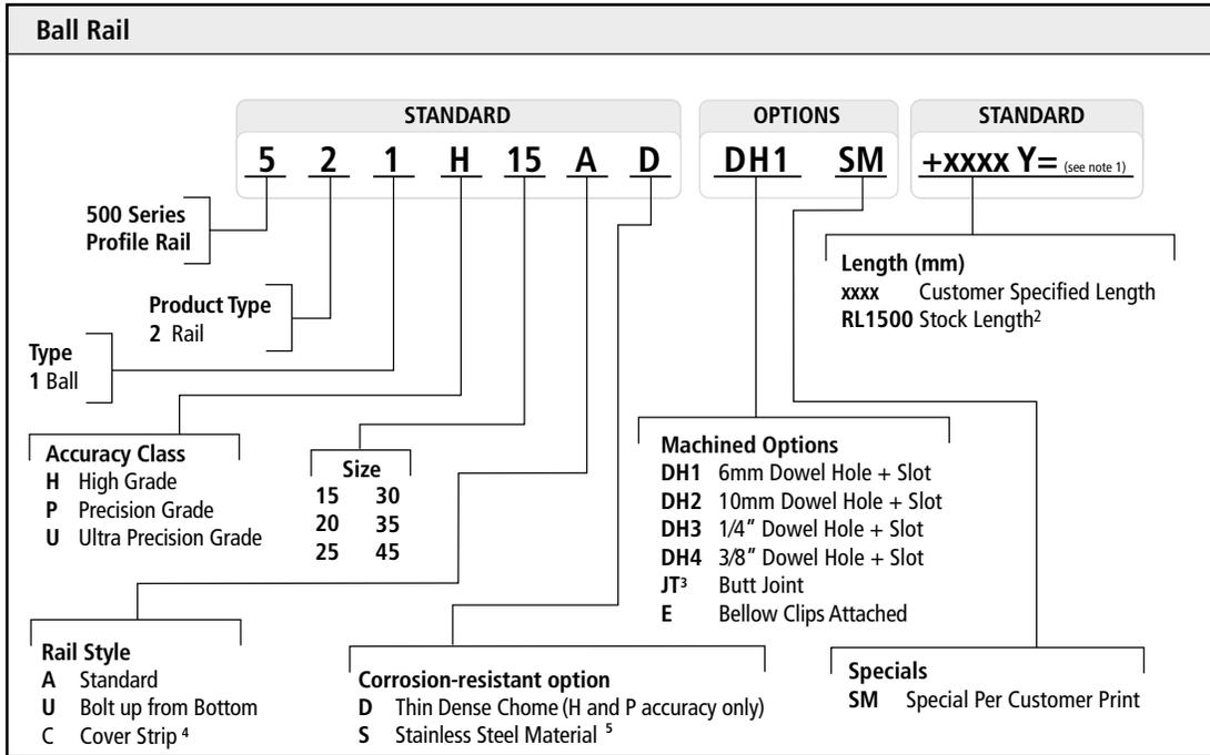
1. Y = Distance from end of rail to center of first mounting hole, Y1 = Y2 unless specified
