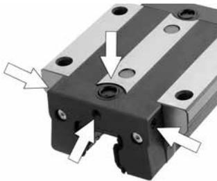
The standard carriage end cap has an integral low friction double lip seal and longitudinal seal that completely encase the bearing carriage. The double lip design keeps contaminants out and lubrication in. It also allows for grease to purge out of the carriage to prevent excessive lubrication, which can result in higher operating temperatures. This double lip design can be used with oil lubrication.
