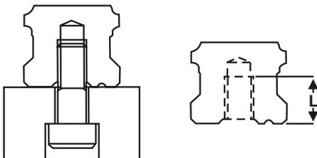
Bolting the rail from the underside allows for a clean top surface with no openings for debris and other particles to collect.
