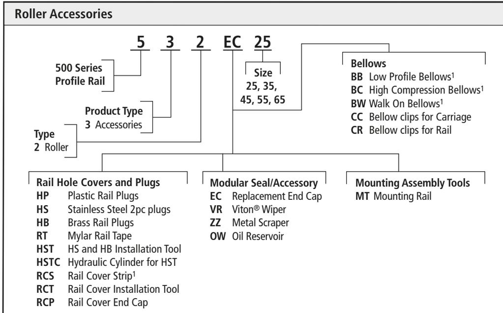
1. Bellows and rail cover strip must include length at time of order. (Example: 532BB35+1000 mm). See page 148 for how to calculate bellows length.
