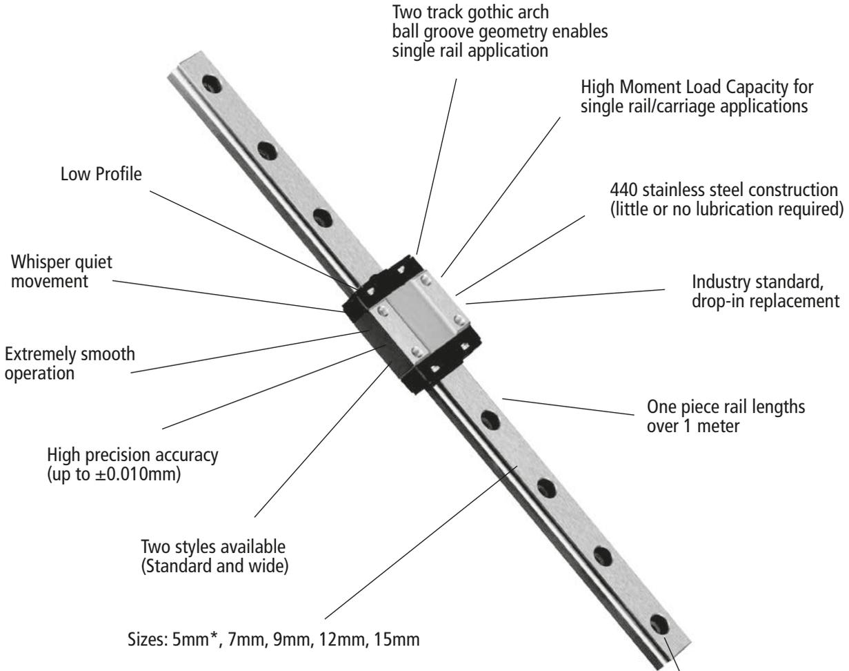
Note! The Microguide linear guide series carriages do not have retained balls. Removing the carriage from the rail without an arbor will result in the balls falling out.
