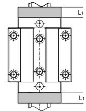
When using a combination of different plates, add the cumulative thickness of the plates to get an accurate overall carriage length.
