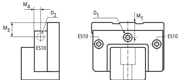
1. D1 and D2 are threaded holes in the end cap to ensure proper integrity and durability of connection.
