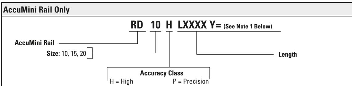
1. Y= Distance from end of rail to center of 1st mounting hole
