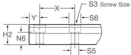
1. "Y" dimension will be equal on both ends unless specified by customer.
