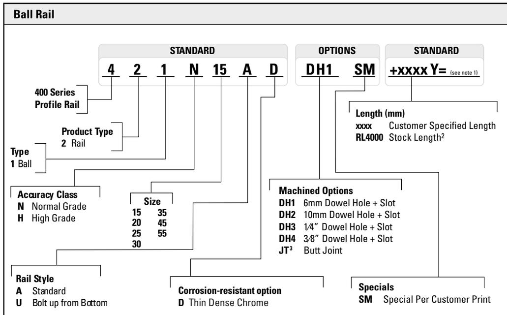
1. Y = Distance from end of rail to center of first mounting hole, Y1 = Y2 unless specified.
