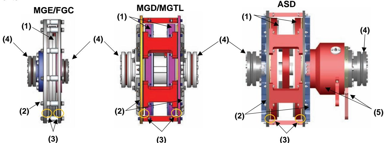
The couplings also have two hubs (4) that are connected to the motor and load shafts with a unique locking mechanism. In addition to all of the components above, the MagnaDrive Adjustable Speed Drives (ASD) also include an actuator mechanism (5) to adjust the air gap spacing between the Conductor Rotor and the Magnet Rotor thus permitting speed control.
