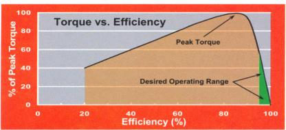
Note: The above torque curve is a generalization of various sizes of magnetic couplings. Coupling selection is based on each application's speed, horsepower, and desired efficiency. Please consult MagnaDrive for proper selection based on your application's requirements
