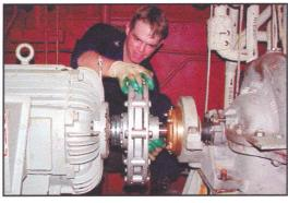
Many of MagnaDrive's couplings are placed on pumping equipment where reliability is critical to ship operations:
