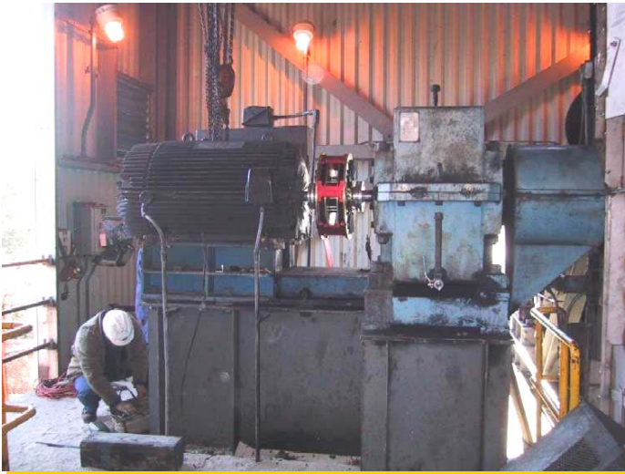
▲ MGTL 18/250, 240HP, 1800RPM, Mining, Conveyor System, UT, USA
