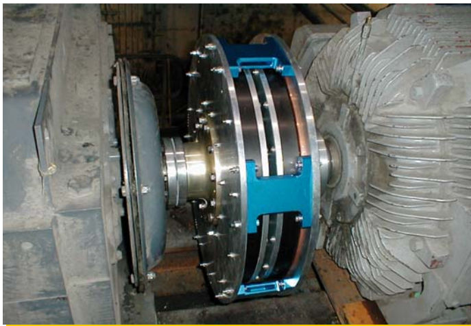
▲ MGD 24/700, 700HP, 1800RPM, Pulp & Paper, Pulper Drum Application, WA, USA
