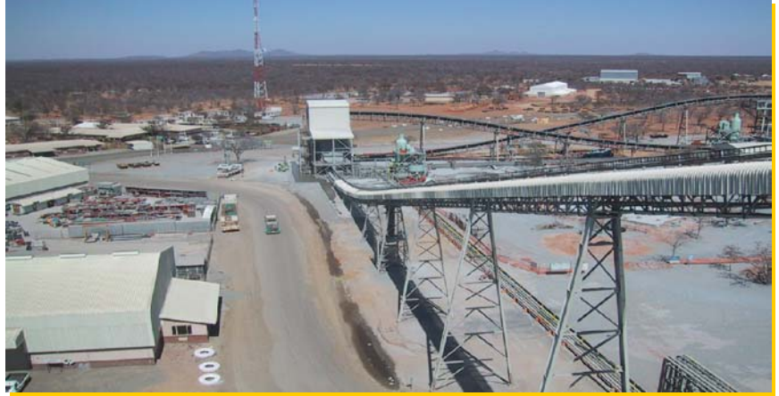
▲ MGD 20/400, 250HP, 1500RPM, Conveyor System, Mining, Botswana
