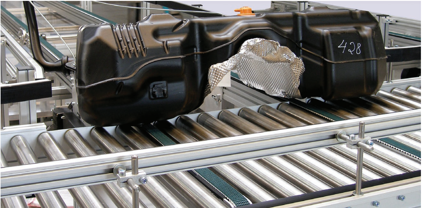
Roller conveyors are ideal for transporting oversized parts. ZRF-P 2010 timing belt conveyors are used to transfer parts between roller conveyors.
