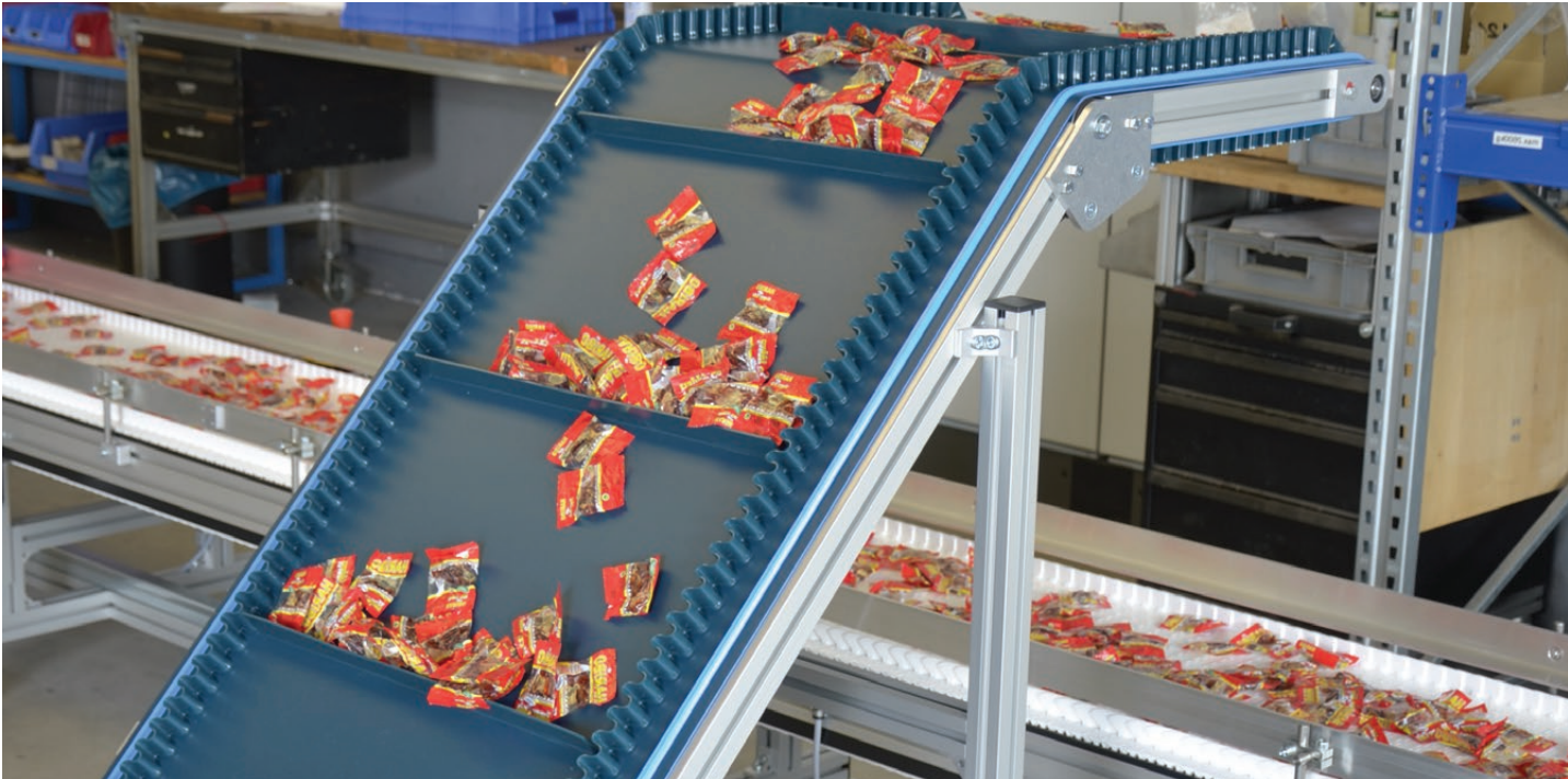
KFG-P 2000 incline to horizontal conveyor feeds product over and onto the conveyor below, which then carries the product downstream.
