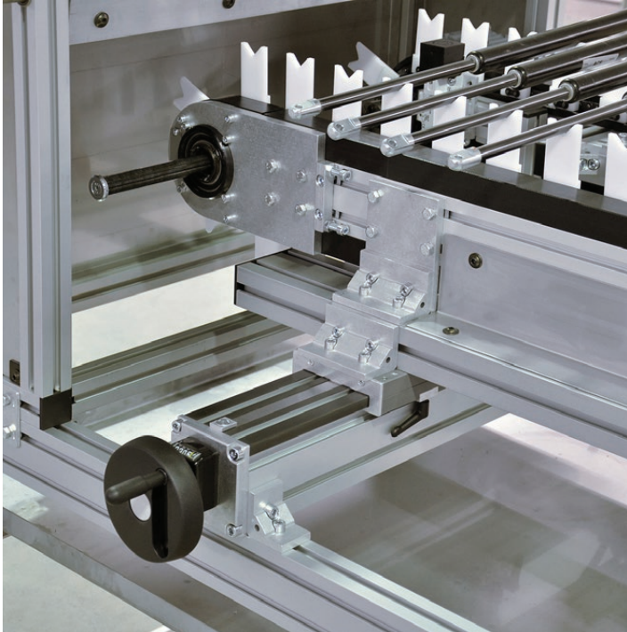
In this example a VST is used to adjust the lane width on an SPU 2040 attachment chain conveyor.
