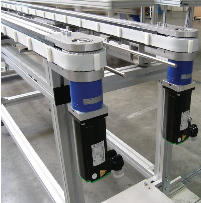
Conveyors can be positioned so that they run on their edges. This can be extremely useful when it is necessary to carry products by their sides.
