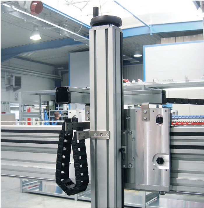
An example of a gantry using an LZR 2005 with a side-carriage and VST 2011 as the Z-axis.
