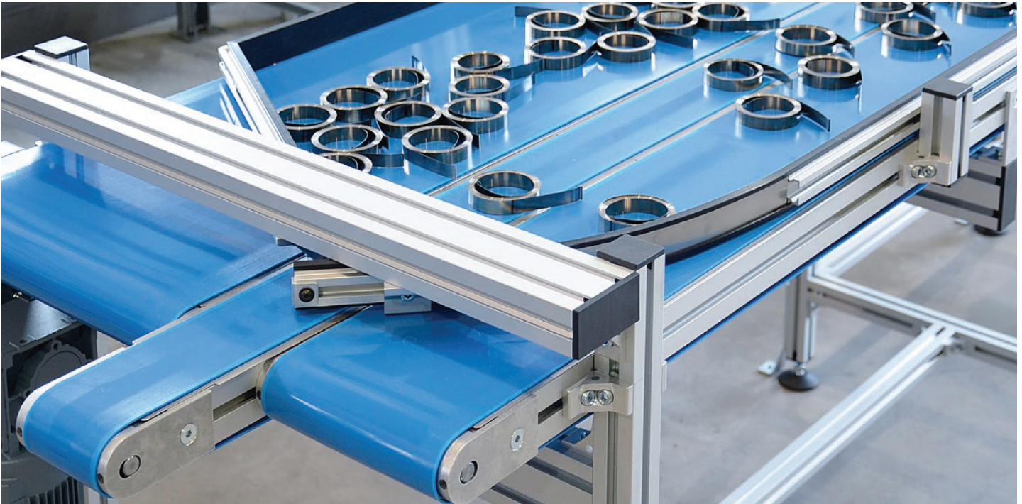
A wide variety of conveyors can be used to accumulate and store parts, including belt conveyors as shown here.
