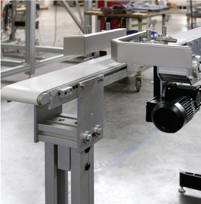
Here a GUF-P MINI conveyor with a center drive is customized with side rails unique for the application.
