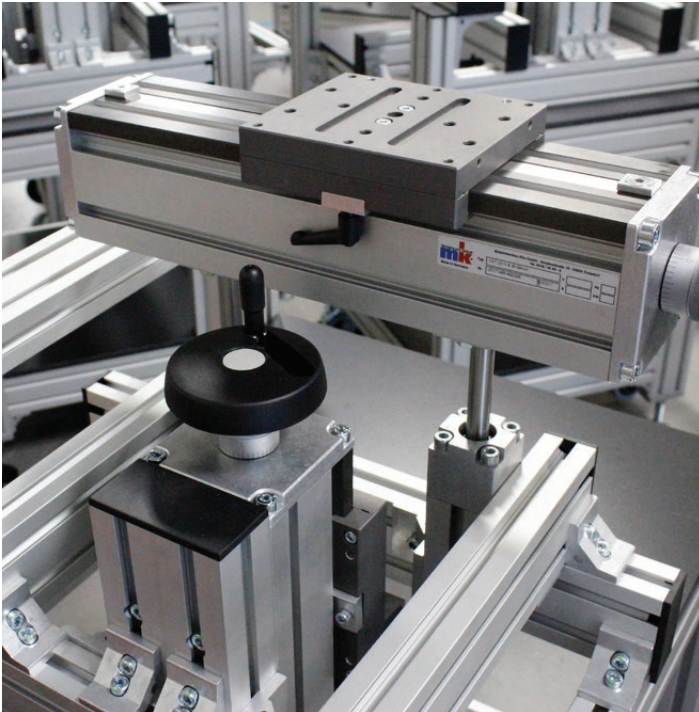
Two VST units are mounted together on a common frame. Additionally the horizontal LZR is also pneumatically actuated.
