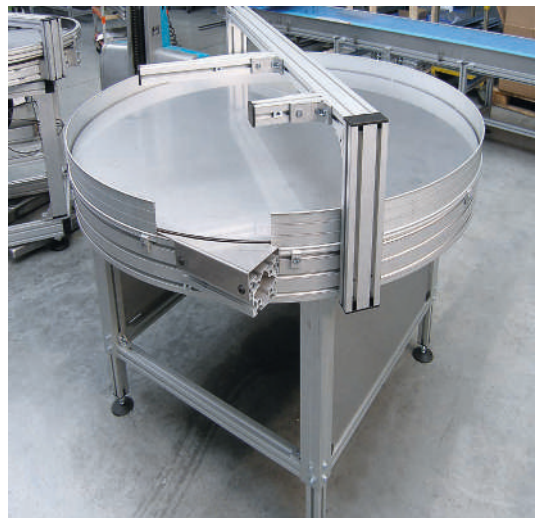
Rotary table with direct drive, stainless steel sheet around the perimeter and single-track discharge
