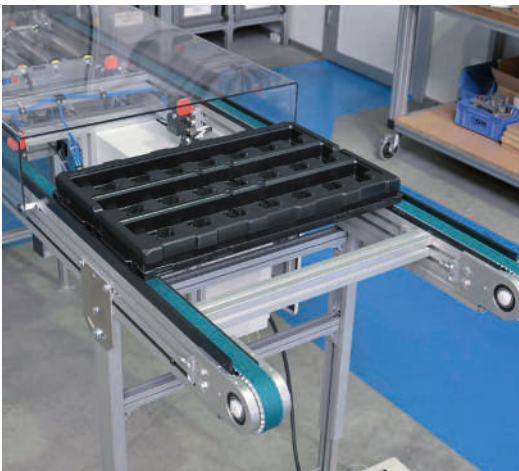
ZRF-P 2010 with stopper/separator function and Makrolon cover as protective guard
