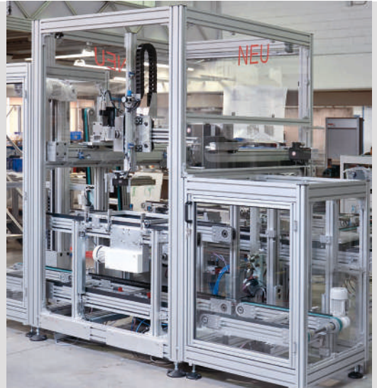
Pallet circulation system for various transport levels with three-axis gantry
