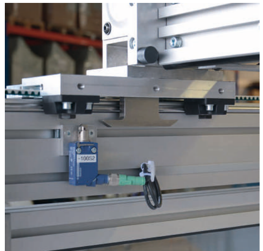
Linear unit LZR 2004-38.41-30 drive coupled via a slip clutch
