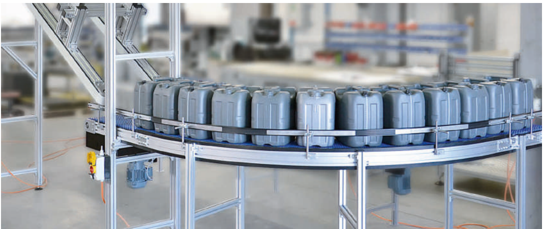
KMF-P 2040 as an infeed for empty canisters
