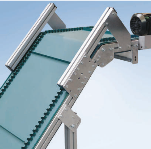
KFG-P 2000 with head drive AU and 45° incline
