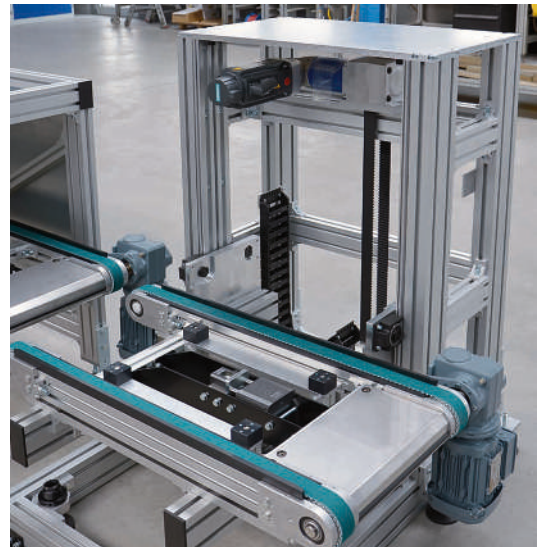
Short stroke lift based on PF-38.44 linear guide system
