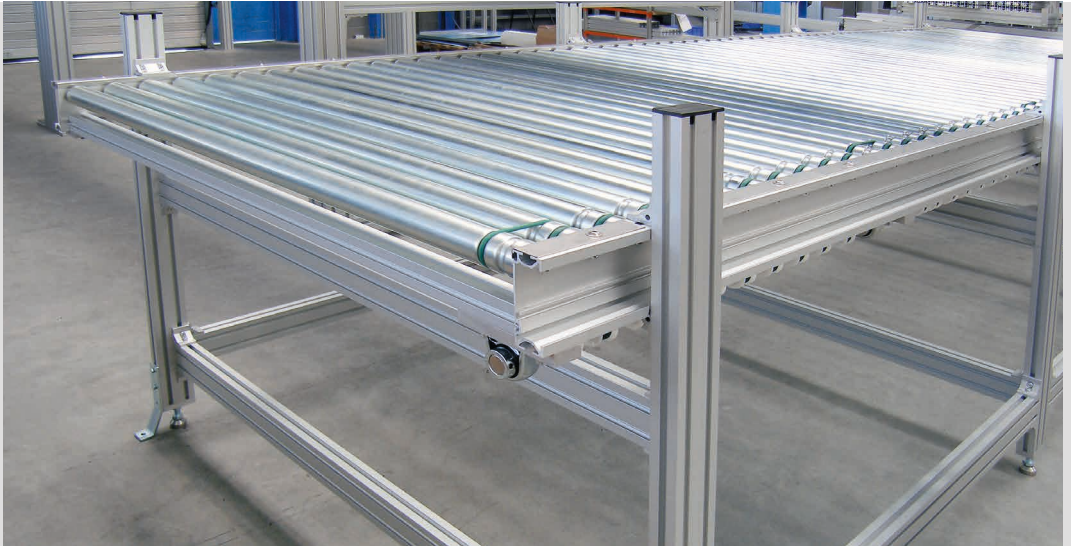
Roller conveyor RBT-P 2066 with vertical shaft drive and diagonal rollers for centring the workpiece on one side
