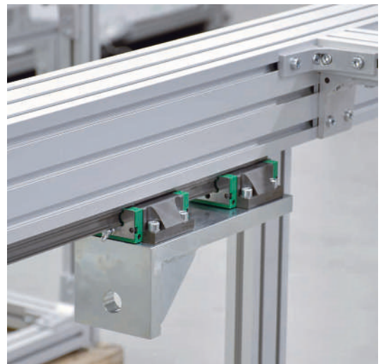
Frame for stress testing based on KU 30.10 recirculating ball bearing guide
