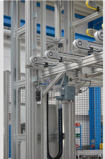
Lift for storage system
