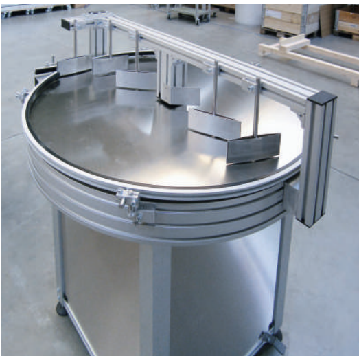
Rotary table with friction belt drive
