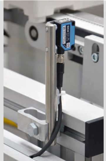
Photoelectric sensor with adjustable holder
