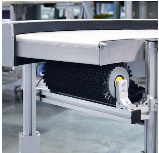
Wiper brush, rotating, mounted at the end of the conveyor
