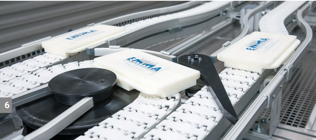
Pallet system based on SBF EMMA A08 with separator
