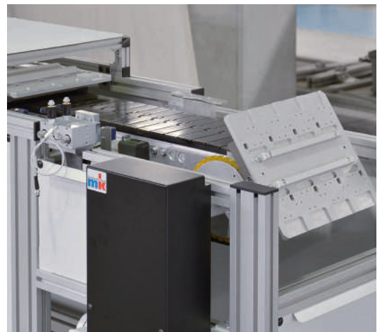
Single-line SPU with custom pallet holder
