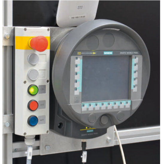
Door dial with emergency stop button and mobile operator panel
