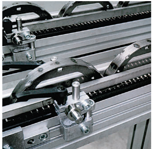
KTF-P 2010 with adjustable side rail and clamp levers for workpieces that frequently change in width
