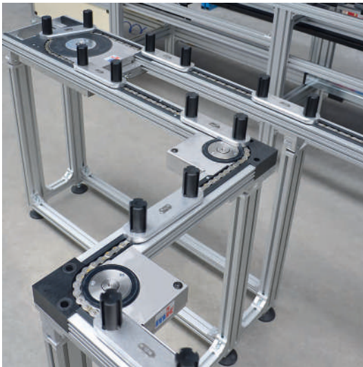
Modu-Con circulation system – the transport medium is a 3/4" vertical hollow pin chain arranged between the wear strips
