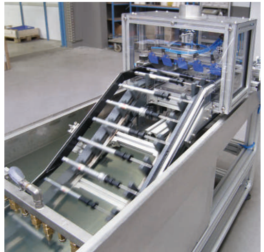
TKU 2040 with 20° inclination and transport of workpieces through a cleansing bath
