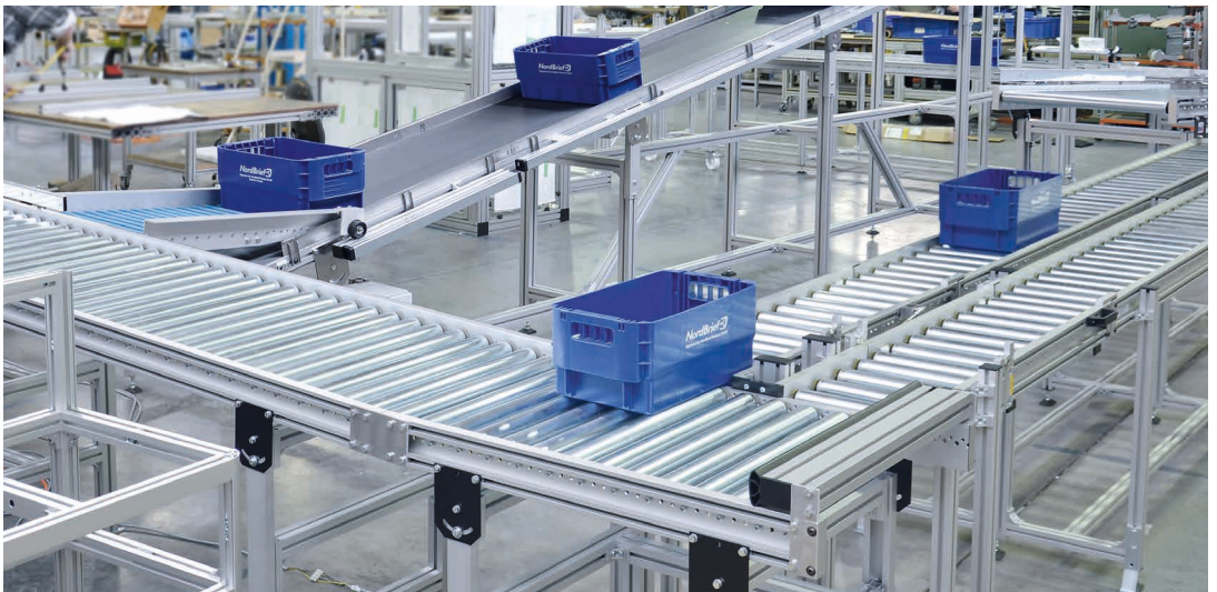
Interlink with RBM-P 2255 driven roller conveyors and RBS-P 2066 gravity roller conveyors for mail crates
