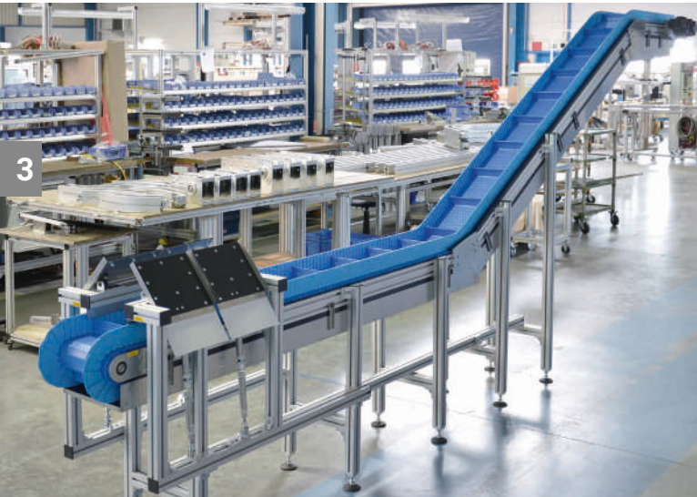
KFM-P 2040 with drip pan and separator flap
