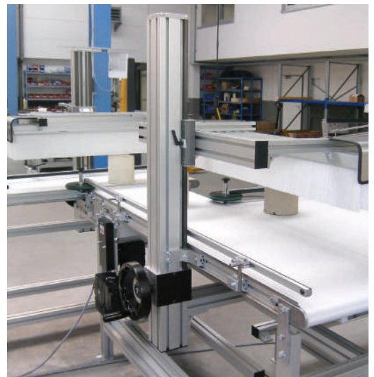
System mk 2011 adjusting unit for brush cantilever
