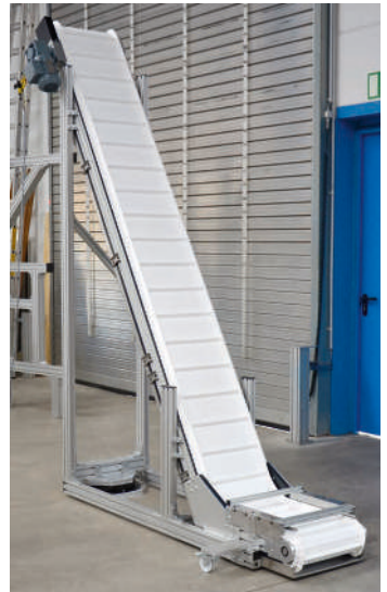
Swivelling KFM-P 2040 with fixed fulcrum, swivel casters and locking mechanism
