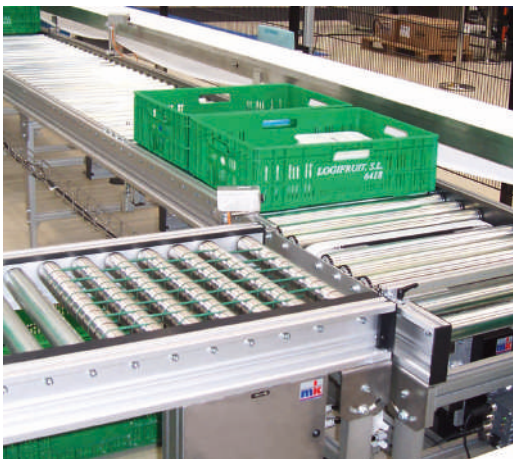
Transport belt combination RBT-P 2255 with integrated lift-and-transfer conveyor
