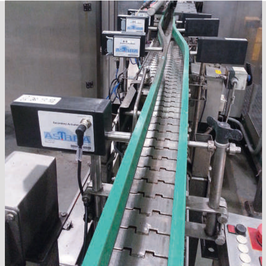
SBF EMMA stainless steel conveyor with automatically adjustable side rail ASTRRA
