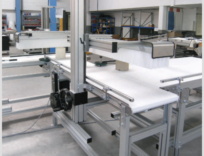
GUF-P 2000 with integrated adjusting unit (VST 2011) for height adjustment of the wiper brushes
