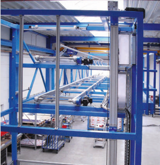
Dual LZR 2005 as lift in steel rack
