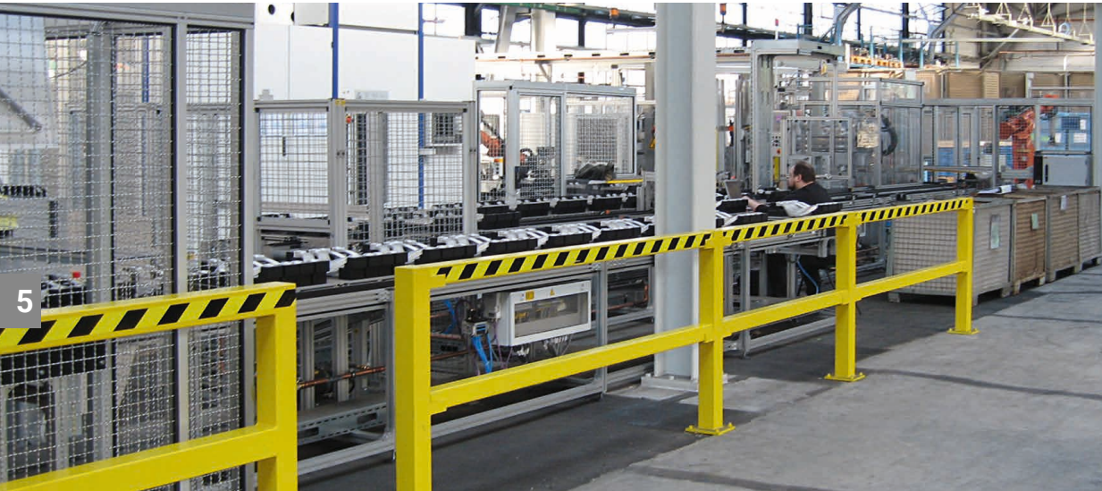
Interlinking production cells in the automotive industry Manual pallet stocking, removal with customer-supplied handling system and robot. Lower return level with lift and shuttle.
