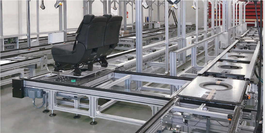
Versamove plus with large custom pallets
