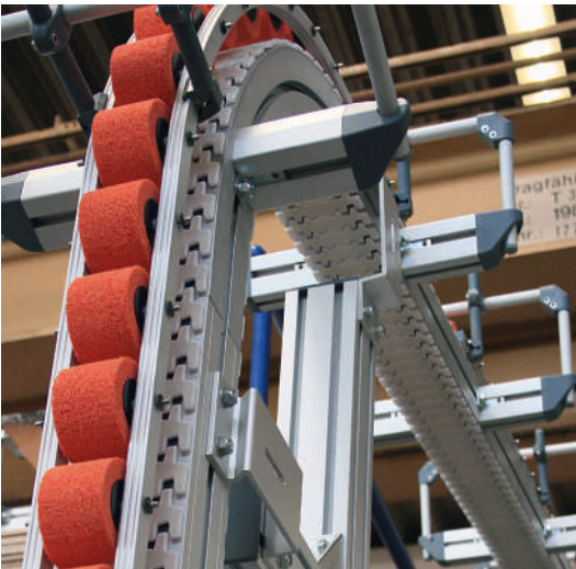
SBF EMMA with pressure rollers for vertical transport
