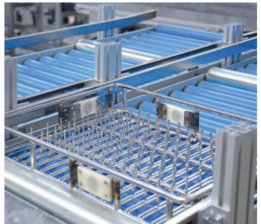
Gravity roller conveyor RBS-P 2065 as feed and discharge conveyor for laundry baskets
