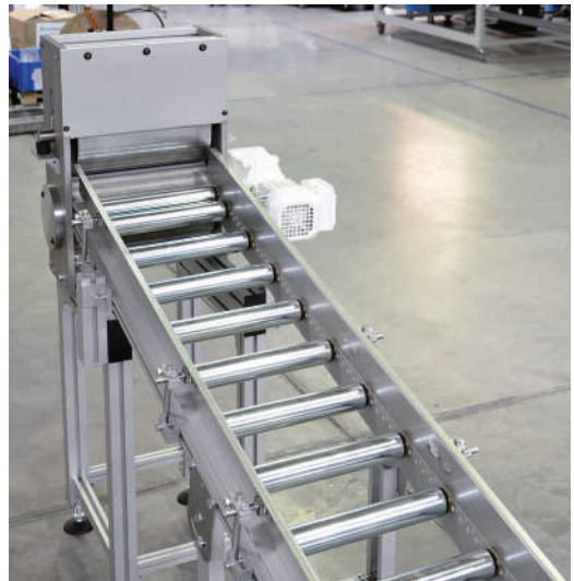
Gravity roller conveyor RBS-P 2065 with 12° incline
