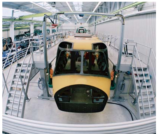
Platform for performing maintenance and assembly work on helicopters safely and with ease
