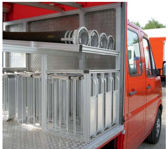
Fire engine interior built from Series 25 profiles
