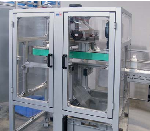
Guarding with swing doors made from cleanroom profiles
