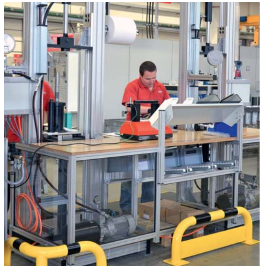
Assembly workstation with integrated press and document holder
