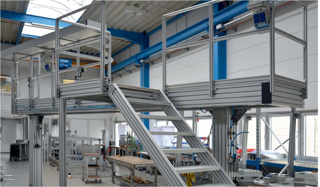
Free-standing assembly platform with 45° stairs
