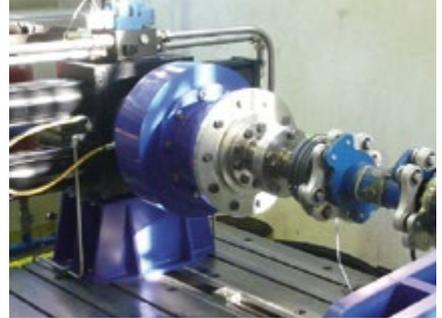
Torque fatigue testing.
