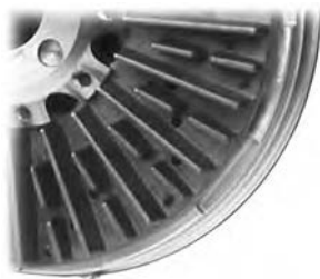
Cross-drilled rotor with heat dissipating fins.
