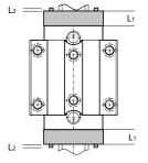
L1 = Lube Block thickness, L2 = max. screw head stickout
