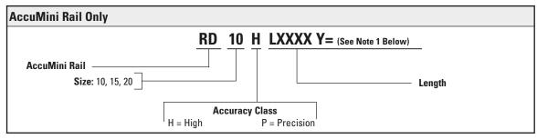
1. Y= Distance from end of rail to center of 1st mounting hole
