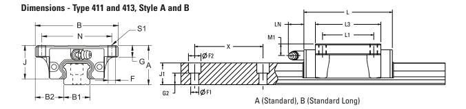
Type 411/413 (No Ball Cage/Ball Cage) - Style A (Standard)
