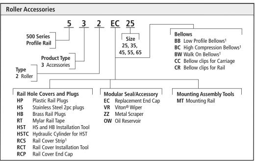
Bellows and rail cover strip must include length at time of order. (Example: 532BB35+1000 mm). See page 148 for how to calculate bellows length.
