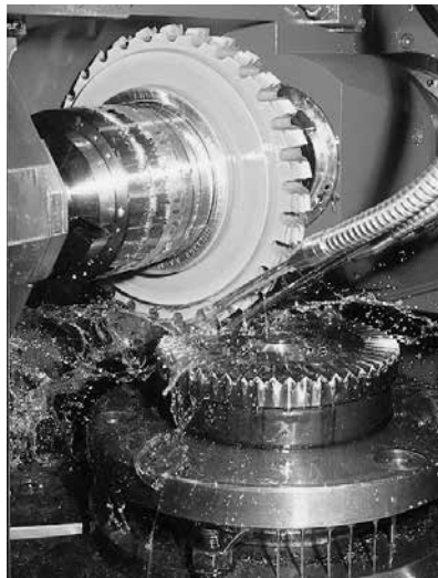
CNC machining of a PowerTRUE right-angle gear
