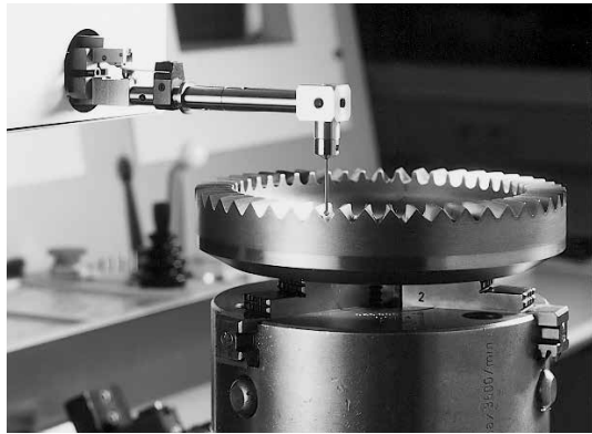
Computerized mapping of gear tooth profile
